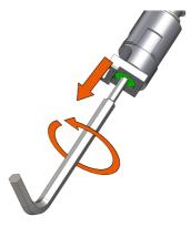
Make sure that the peeler blade lies flat on the blade holder and that it touches the stop with its backside.
