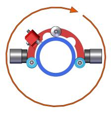
Watch how the chip is removed. If the peel width is maximum 2/3 of the blade width continue moving the U-Peeler around the pipe until you have scraped the desired area of the pipe surface.
